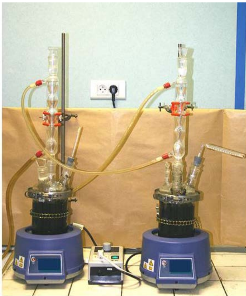
Figure 2.16.4—a Example of testing equipment available on the market to perform UN Test C.1
